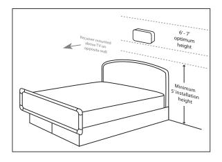
The transmitter must be mounted a minimum of 5 feet above the floor with 6-7 feet being optimal. The speaker must be mounted above the bed and at least 5 feet above the floor with 6-7 feet being optimal.
